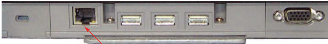
Docking station terminal strip (arrow pointing to RJ45 port)
